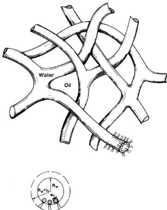
**Fig. 1.** A model structure proposed by Ninham, Evans and coworkers for a conductive bicontinuous microemulsion formed in low water content water-DDAB-isooctane systems [3].
