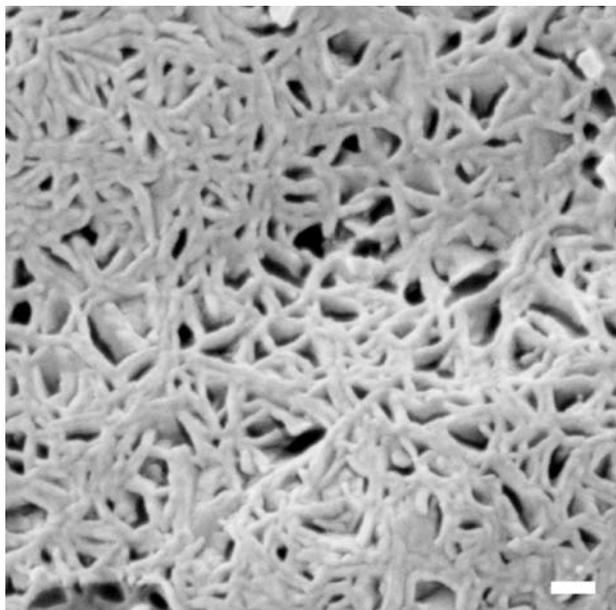
**Fig. 2.** A cryo-SEM micrograph of a 48%/32%/20 wt% isooctane/DDAB/water microemulsion; bar = 100 nm.
