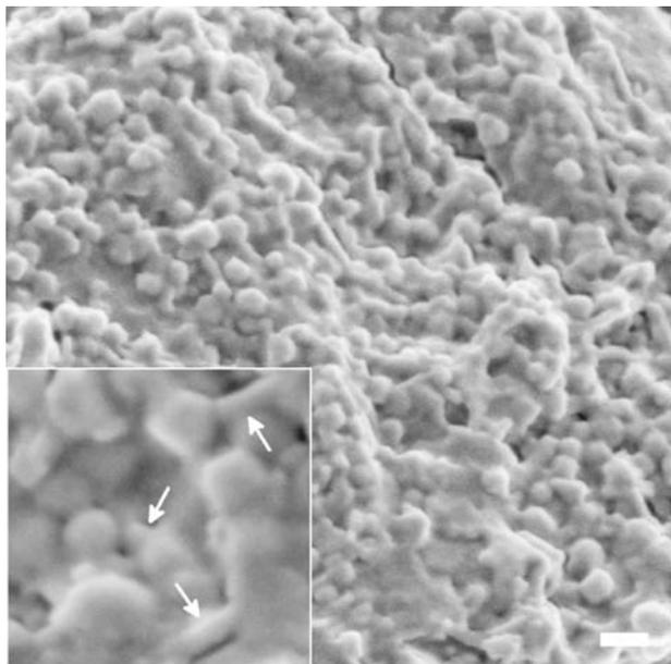
**Fig. 5.** A cryo-SEM micrograph of a 42%/28%/30 wt % isooctane/DDAB/water microemulsion; bar = 100 nm. Inset – doubled magnification. Arrows indicate conduits connecting inverse swollen micelles.
