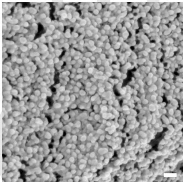
**Fig. 4.** A cryo-SEM micrograph of a 36%/24%/40 wt % isooctane/DDAB/water microemulsion; bar = 100 nm.
