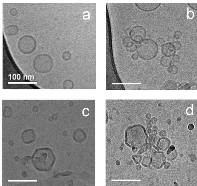
Fig. 7. Cryo-TEM images of liquid DOPC/POPS<sup>1-</sup> liposomes (a), solid DPPC/POPS<sup>1-</sup> liposomes (c) and their complexes with the SPE (b and d, respectively).  $\nu = 0.1$ ; [SPE<sup>+</sup>] = 10<sup>-4</sup> M; total lipid concentration 2 mg/mL.
