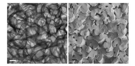
Fig. 5 Cryo-EM micrographs of the system, 7 wt%  $C_{12}E_5$ , at  $\alpha$ =40 % and 34 °C (**a**, **b**), and 60 % and 36 °C (**c**, **d**). The micrographs shown in **a** and **c** are of cryo-TEM, and those in **b** and **d** are cryo-SEM. *Bars* are 200 nm (**a**), 500 nm (**b**), 200 nm (**c**), and 400 nm (**d**)
