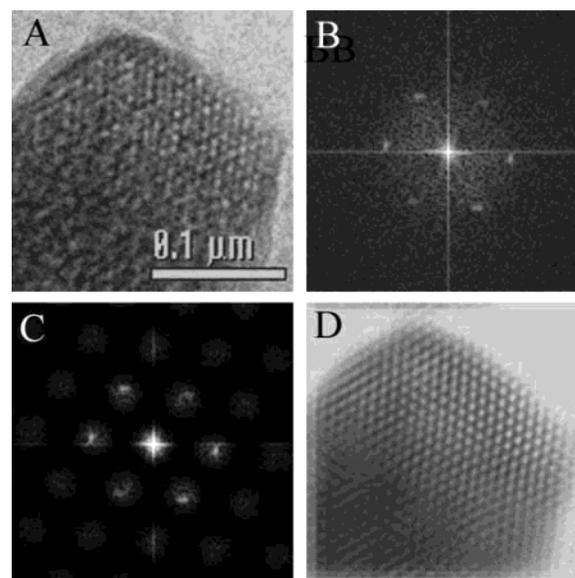
**Figure 5.** Digital filtering of a cryo-TEM image and complex aggregate at  $r = 13.3$ . (A) Original, unprocessed digital image. (B) Fast-Fourier transform (FFT) of image A. (C) Filtered FFT of the transform of image B. (D) Inverse transform of image C, i.e., the filtered imaged of the original micrograph.
