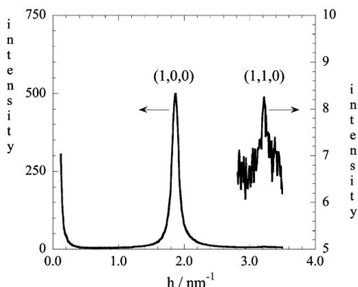
**Figure 7.** SAXS patterns from SDS–PDAC complex dispersion after drying. The initial dispersion contained 0.1% PDAC at  $r = 1$ .
