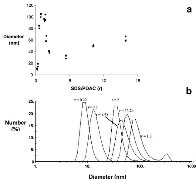
**Figure 1.** (a) Light scattering results showing average diameter of particles as a function of SDS/PDAC molar ratio. PDAC final concentration in all samples is  $6.8 \times 10^{-3} \text{ M}$  (based on the monomeric unit) SDS concentration is varied from 1.5  $\times 10^{-3}$  to 0.2 M. Duplicate results are shown for each  $r$  ratio. (b) Size distribution of SDS–PDAC aggregates at different  $r$  ratios.
