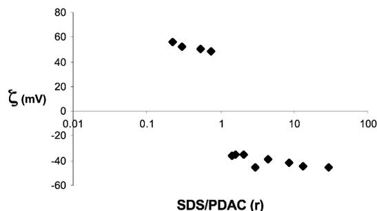
**Figure 2.** Zeta potential ( $\zeta$ ) of SDS–PDAC particles as function of the SDS/PDAC molar ratio,  $r$ . PDAC concentration fixed at  $6.8 \times 10^{-3}$  M (based on the monomeric unit); SDS concentration is varied from  $1.5 \times 10^{-3}$  to 0.2 M.
