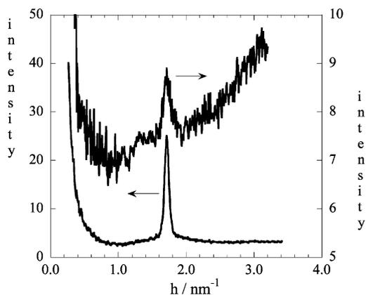
**Figure 6.** SAXS patterns from SDS–PDAC complex dispersion from 0.1% PDAC solution at  $r = 0.9$  (top) and  $r = 13.3$  (bottom).
