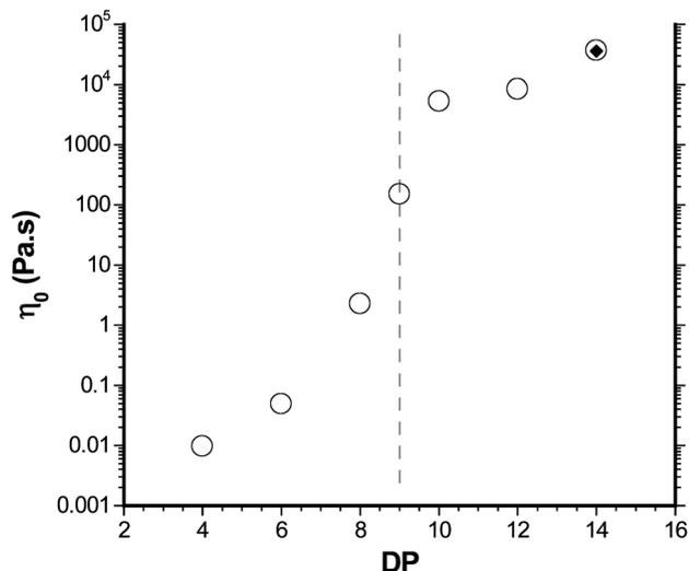
**Fig. 6** Semi-log plot of zero-shear viscosity  $\eta_0$  as a function of DP. The closed rhombus corresponds to the sample DP14 formulated with DCFH. The vertical dashed line indicates a rough transition between sol- and gel-vesicle systems.
