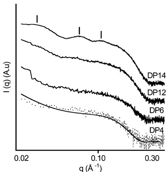
**Fig. 1** log-log plot of SAXS patterns collected at 25 °C of the samples DP4, DP6, DP12, and DP14. Curves are shifted for clarity with multiplication factor 5. The dotted line in DP4 represents the experimental curve with the superimposed fitting curve (continuous line) obtained with GAP analysis.
