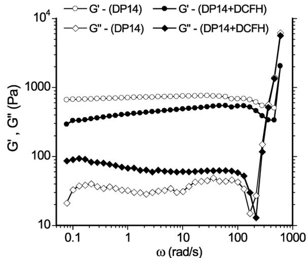
**Fig. 7** Linear viscoelastic experiments at 25 °C for DP14 sample (open symbols) and DP14 sample loaded with diclofenac DCFH (closed symbols). Circles: storage modulus  $G'$ ; diamonds: loss modulus  $G''$ .
