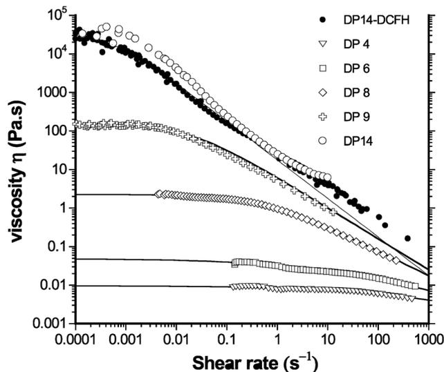
Fig. 5 log–log plot of shear viscosity vs. shear rate measured in steady state experiments as a function of DP. The solid lines are the best fits of eqn (2).
