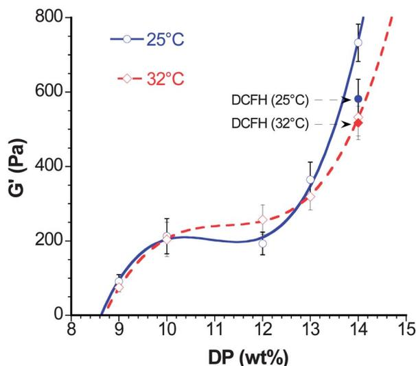
**Fig. 8** Storage modulus  $G'$  as a function of DP compositions at two different temperatures.  $T = 25\text{ }^{\circ}\text{C}$ : open circles with the solid line as guide for eyes; the closed circle corresponds to DP14 gel vesicles encapsulating DCFH.  $T = 32\text{ }^{\circ}\text{C}$ : open diamonds with the dashed line as guide for eyes; the closed diamond corresponds to DP14 gel vesicles encapsulating DCFH.
