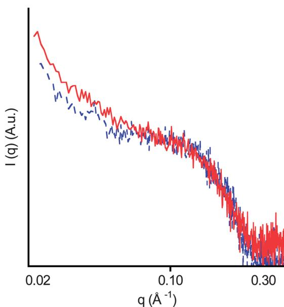
**Fig. 3** log-log plot of SAXS patterns collected at 25 °C of the VLG diluted sample (dashed line) of composition MO/LCh/W = 3.3/0.3/96.4 (wt%) compared with the DP4 sample (solid line) having the same nominal composition.
