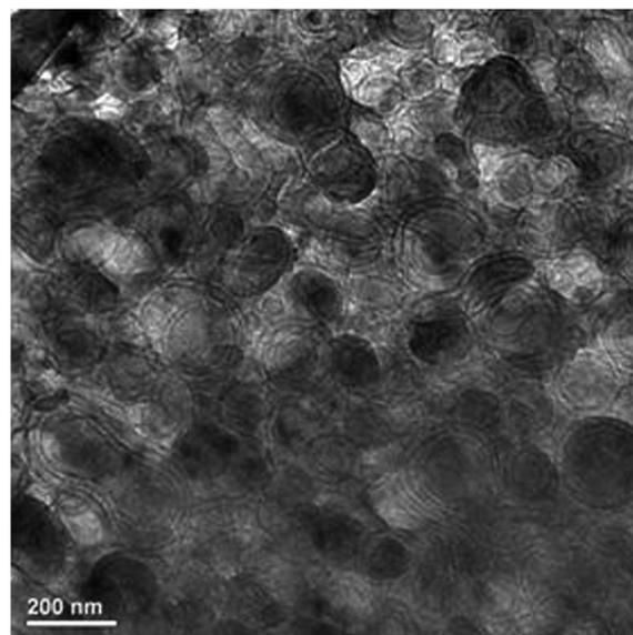
**Fig. 2** Cryo-TEM image of the VLG sample DP14 with composition MO/LCh/W = 13.2/1.2/85.6 (wt%) showing oligo-lamellar close-packed vesicles.
